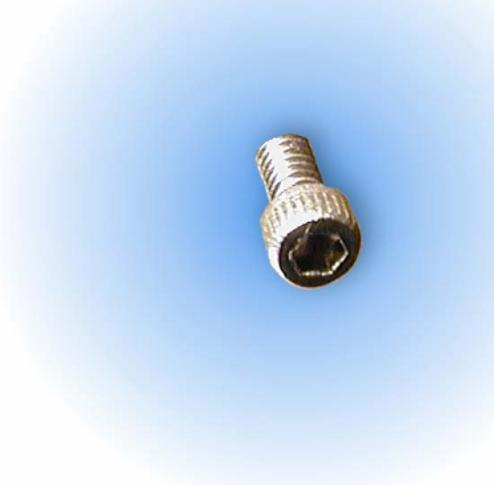
This bolt holds the selector lever on its shaft.
