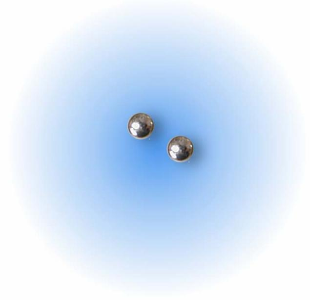
Hard steel ball bearing used as the safety detent.
