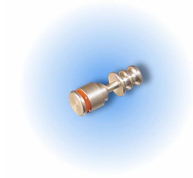
If you are able to see the red line the marker is off safe and will fire. Be careful when removing this shaft; there are springs and ball detents in the frame.
