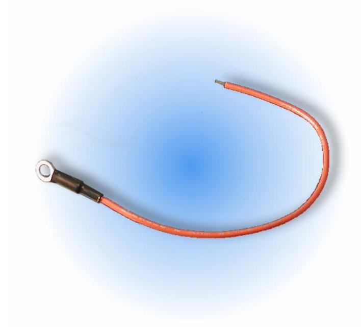
The power wire from the battery contact bolt in the front of the grip frame to the PC board.
